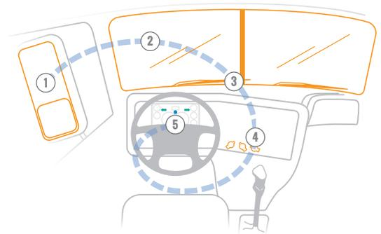
**Safe Start.** Tell the examiner these 3 steps before you perform them: parking brake is set, transmission in neutral, and the clutch is depressed. Start the engine and look for the **ABS light** on the dash to come on and then go off. With the vehicle started, check the gauges.
