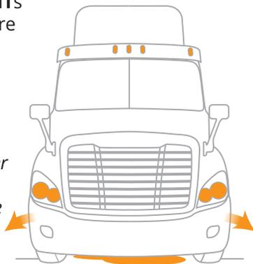
**Coolant:** verify proper level, not leaking, securely mounted, not BBC; check the **hoses** for splits or cuts and ensure they are securely mounted.
